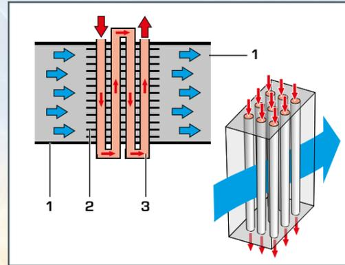
1 air duct, 2 fins, 3 water pipe section,
