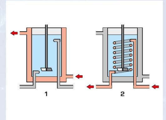
1 heating via the jacket, 2 heating via the coiled tube
