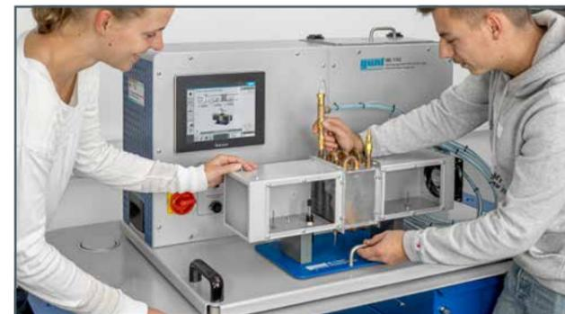
3. Attach the hose connection to the finned tube heat exchanger.
