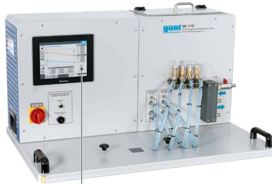
Connection to max. 10 mobile end devices via integrated WLAN router
