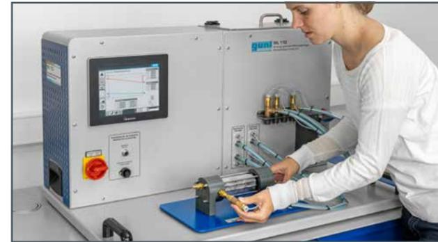
1. Remove the hose connections on the shell and tube heat exchanger.
