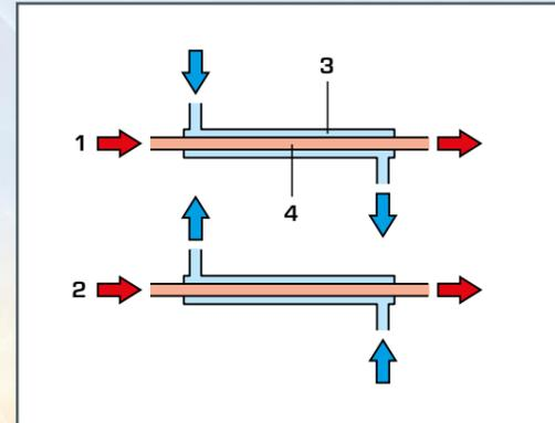
1 parallel flow operation, 2 counterflow operation,
