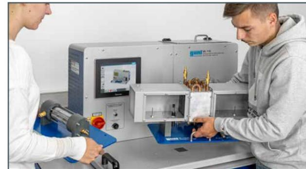
2. Remove the accessory and replace it, no tools needed. Position the finned tube heat exchanger on the work surface of the supply unit.
