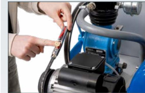
Checking the belt tension
