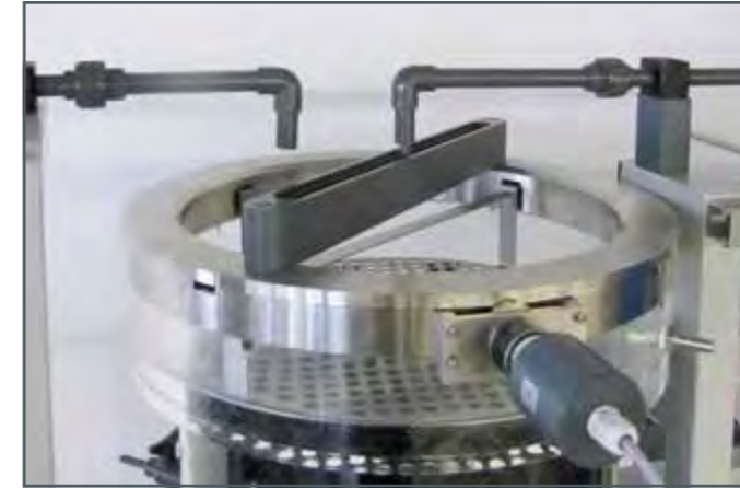
Rotary distributor on the head of the trickling filter with variable speed adjustment
