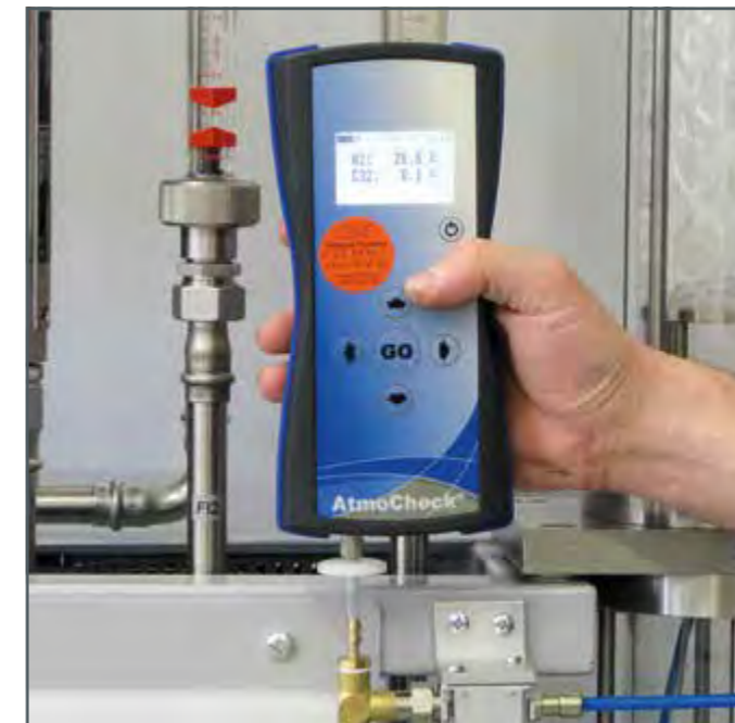
Gas analyser for determining the oxygen content and carbon dioxide content.
