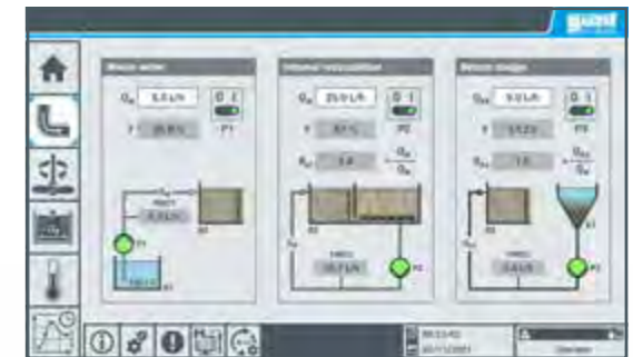
Touch screen: operation of the pumps
