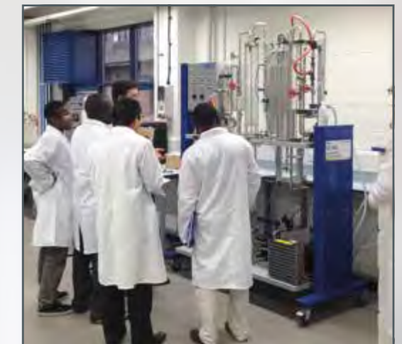
A GUNT employee explains the functional principle of CE400 gas absorption to lecturers at the University of Hull.
