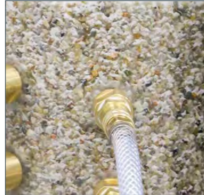
By using a transparent filter tube, you can also observe the increased loading of the filter bed visually as well as using the rise in pressure loss.
