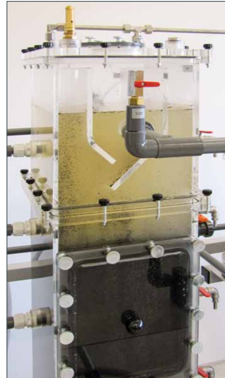
CE 702's UASB reactor during a successful trial run in our laboratory
