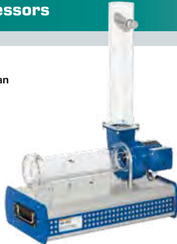
HM 292 Experiments with a radial compressor Two-stage compressor: recording of the compressor curve for both stages
