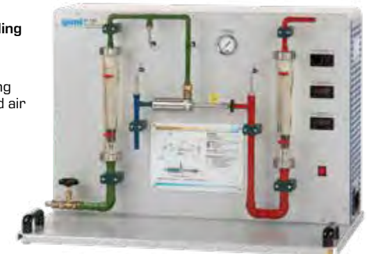
ET 480 Absorption refrigeration system Thermally driven refrigeration system without compressor that can be heated with either gas or electrically
