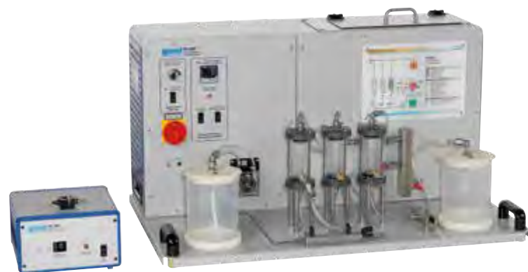
CE 584 Advanced oxidation Oxidation of organic substances with hydrogen peroxide and UV light
