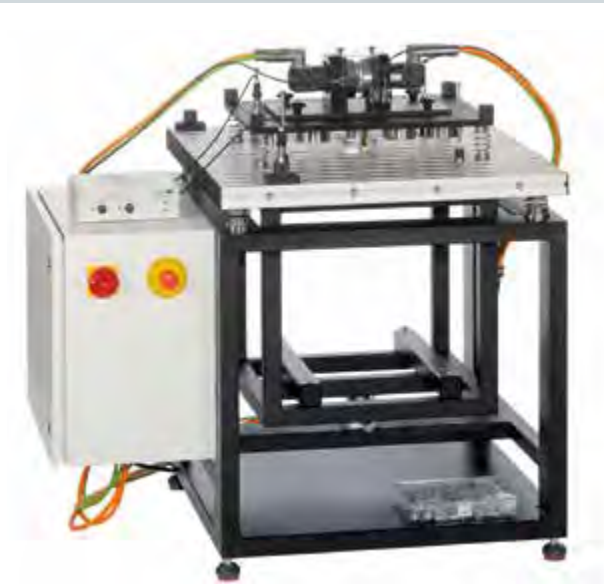
TM 182 Vibrations on machine foundations Machine foundation and isolation of vibrations
