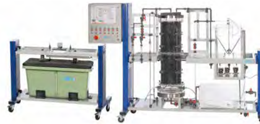
CE 704 SBR process Sequencing batch reactor
