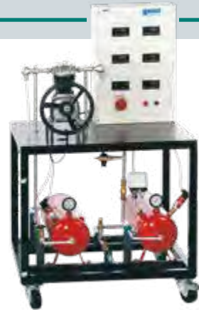
ET 513 Single-stage piston compressor Investigations on an air compressor including the determination of the mechanical power consumption
