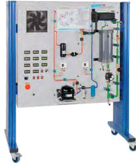
ET 120 Cooling using the Peltier effect Demonstration of the thermo- electric effect
