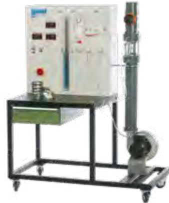
HM 210 Characteristic variables of a radial fan Determination of flow rate via iris diaphragm or Venturi nozzle
