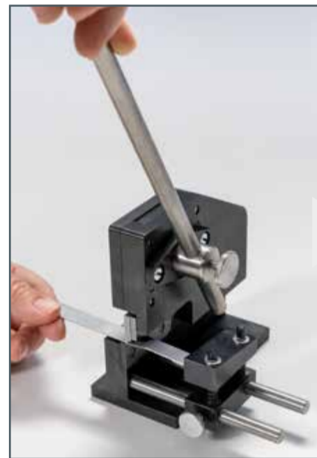
Cutting sheet metal with the lever shear from TZ 200.07
